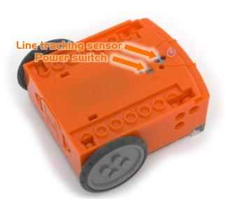
Edison's power switch and line tracking sensor
