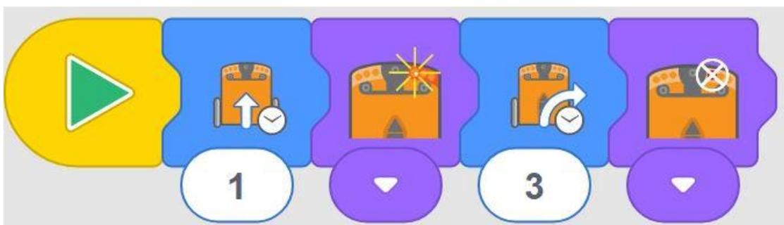
In this activity, to get Edison to drive forward a set distance, students need to select the action of ‘drive forward’ with the time controlled duration, then experiment with the amount of time they input to get Edison to drive the correct distance.
