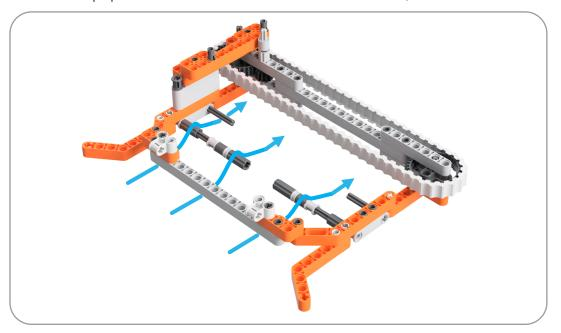
The paper should first go under the front grey beam. It then needs to go over the longer set of bars with the rollers attached. The paper should sit between these rollers and the paper-controlling Edison's wheels. Finally, the paper should be slid under the short set of axles protruding from the frame of the EdPrinter. These axles keep the paper in place.
