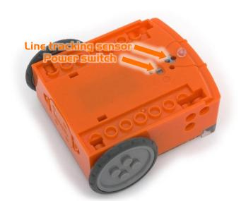
Edison's line tracking sensor is made up of two parts: a red LED light and a light sensor.
