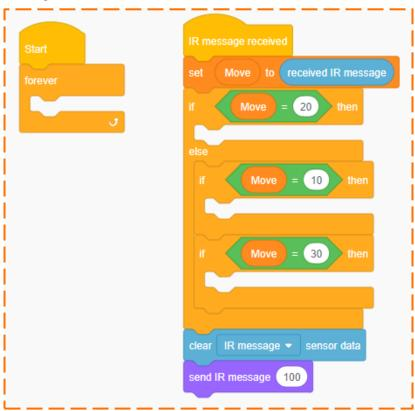
This isn't a full program, but you can use this code to help you build your driver bot program. This section of code uses a variable called Move. The value of this variable is set to be whatever the value of the received IR message is. When you work with sensor values, you should always store any values you want to use in your program in a variable. You can then have your program use that variable in whatever ways you need anywhere in the program.
