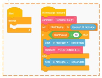
This isn't a full program, but you can use this code as an example to help you build your performer bots' programs. This section of code uses a variable called StartPlaying. The value of this variable is set to be whatever the value of the received IR message is. When you work with sensor values, you should always store any values you want to use in your program in a variable. You can then have your program use that variable in whatever ways you need anywhere in the program.
