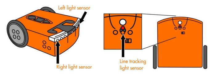
Much like Edison's infrared receiver can detect infrared light, the light sensors can be used to detect visible light, which is the portion of the light spectrum that people can see. All of Edison's visible light sensors work basically the same way as the light sensor in Edison's line tracker works when you use it to detect reflective and non-reflective surfaces under the robot.
