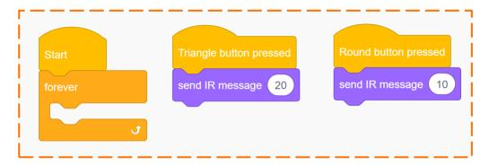
You can use this as your controller bot program. This program tells the Edison acting as the controller bot to send out an IR message whenever you press the round or triangle button on the controller bot. If you press the triangle button, the controller bot will send out IR message 20. If you press the round button, however, the controller bot will send out IR message 10 instead.
