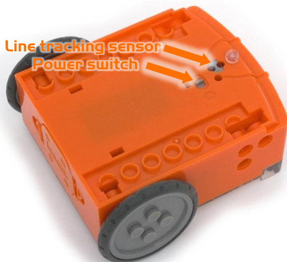
Edison's power switch and line tracking sensor
