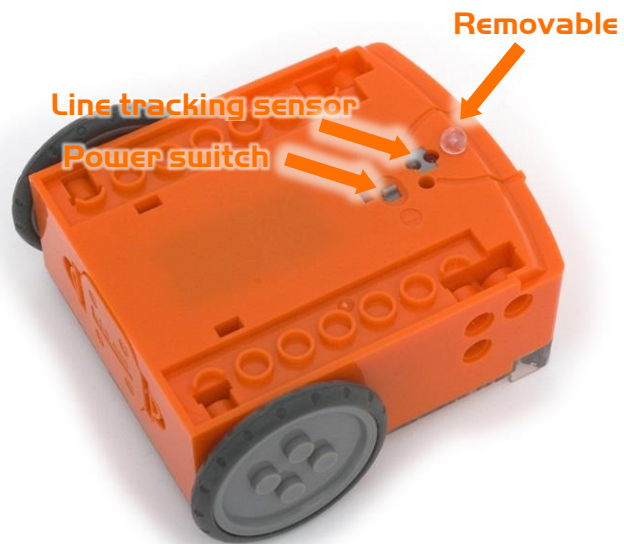
Location of Edison's power switch, skid, and line tracking sensor.
