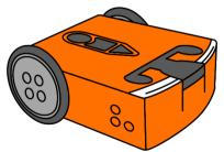
There's a lot we can do with our Edison robots. We can program the robot to do things like drive using its motors, flash its LED lights or make sounds. Edison also has different sensors which we can use to get the robot to behave in different ways.
